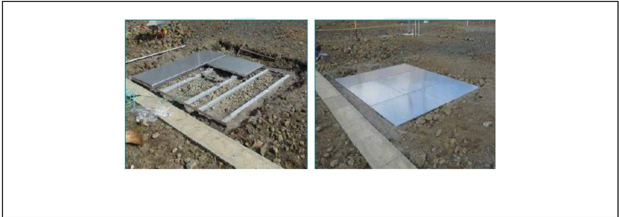
Figura 3-7: Sensor SSG Snow Scale
